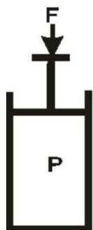
Figure 4.2 (left): Illustration of the force on a piston determining the pressure in a cylinder.
